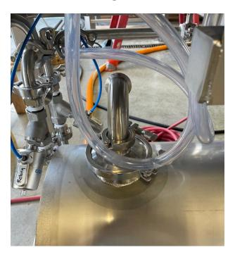
Mix your preferred cleaning chemicals into the 15gal caustic reservoir. Pour and mix into the 4" port on the top of the reservoir. Attach the overflow vent cap when done.
